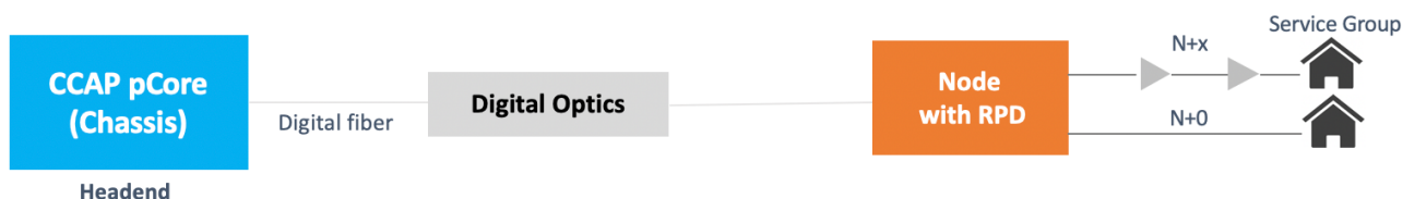
Figure 4. Remote PHY with Hardware CCAP Core
