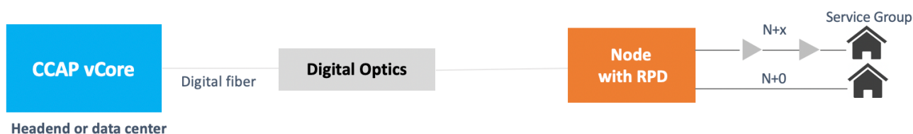
Figure 5. Remote PHY with Virtual CCAP Core
