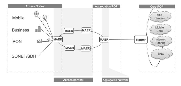
Figure 2. Super-Converged, Multi-Access Edge Network for Mobile, Business, Residential, and SONET/SDH Transport Services
