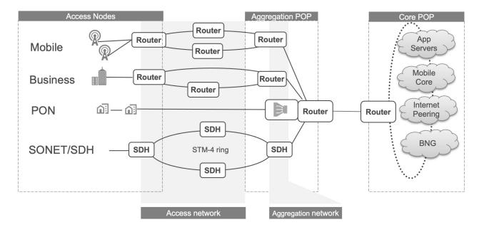
Figure 1. Many Network Operators Run Parallel Access Networks for Different Services
