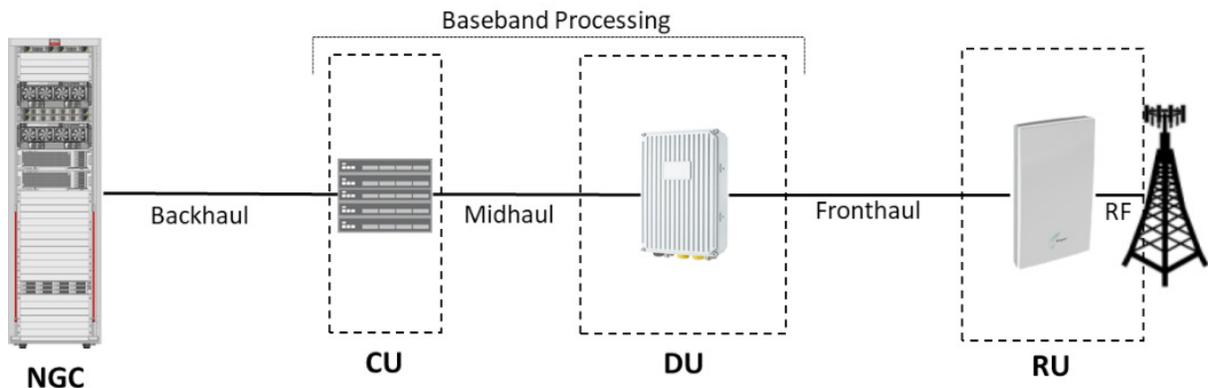
**Figure 1. Adding Fronthaul and Midhaul Links to Backhaul in Transport Networks for the 5G RAN**
