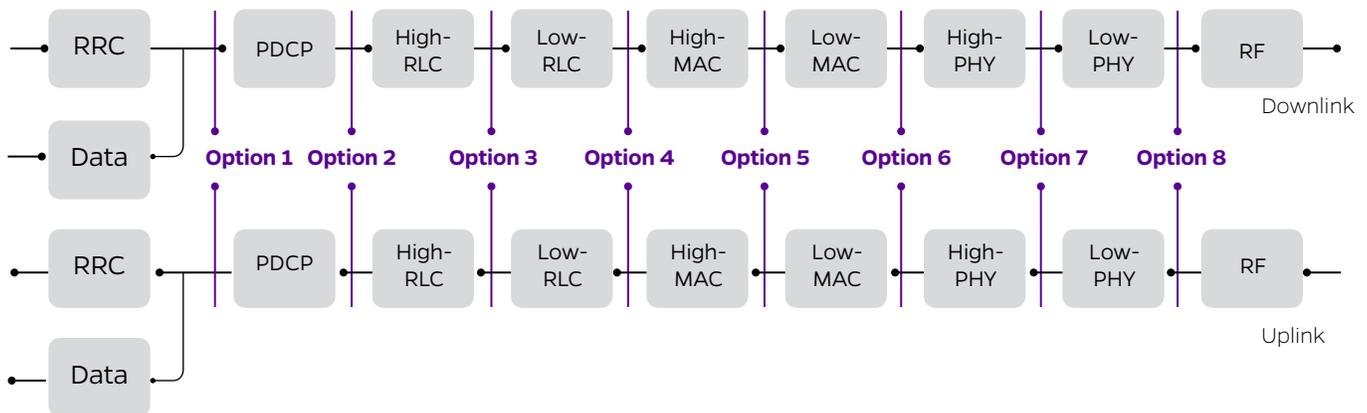
*Figure 3. Options for Implementing the Radio Protocol Splits in xHaul Designs*
