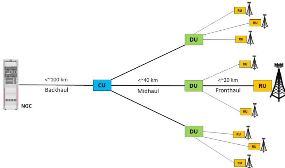
*Figure 4. Aggregation of Midhaul and Fronthaul Connections*
