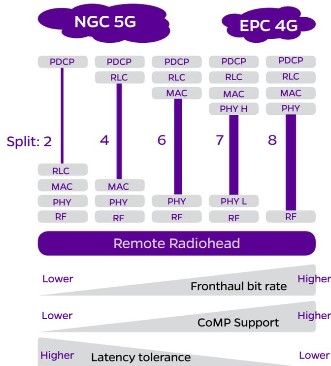
Figure 2. Radio Protocol Processing Splits and the Transport Networking Configurations They Create
