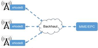
Figure 2. 4G/LTE RAN Backhaul to Mobile Core
