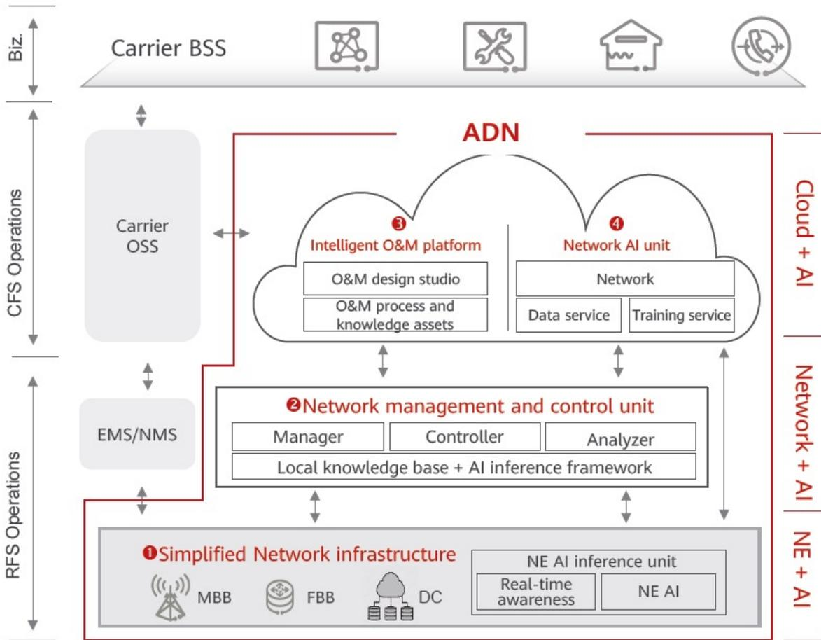
**Figure 3. Huawei ADN Network Solution (Source: Huawei, 2020)**
